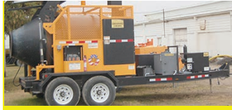
2014 Asphalt Reclaiming Tumbler Diesel Fired, Hydraulic Controlled, Rotation 9RPM, 3/16" Steel 450 Brinell Hardened Drum, (7) 3/16" 450 Brinell Hardened Agitation Paddles, 80 Gal Fuel Tank, Produces 4 Tons/ Hour, 50hrs, Use Year Round 989-777-4550 sales@spauldingmfg.com
