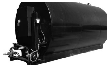
A000 Gallon Sealer Bulk Tank, gas engine, belt drive Viking pump and off-center mixer. Cleanout cover, used for last 35 years consecutively, 16' long x 8' diameter. Call Fred at 216-341-0883 (x/G-21)
