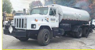
1992 Etnyre Distributor Sam-2 , International with 3,730-gallon tank with diesel burners, 165,652 miles, 18 ft spray bar, runs good. $20,000 814-764-5080 x107 (x/E-21)
