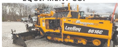
2017 LeeBoy 8616 Kubota 111 HP Diesel Engine with 8-15' Legend Electric Screed. 9 Ton Conveyor Hopper and Poly Pads. SLOPING SCREED EXTENSIONS HEATED ENDGATES Power Crown $110,000
